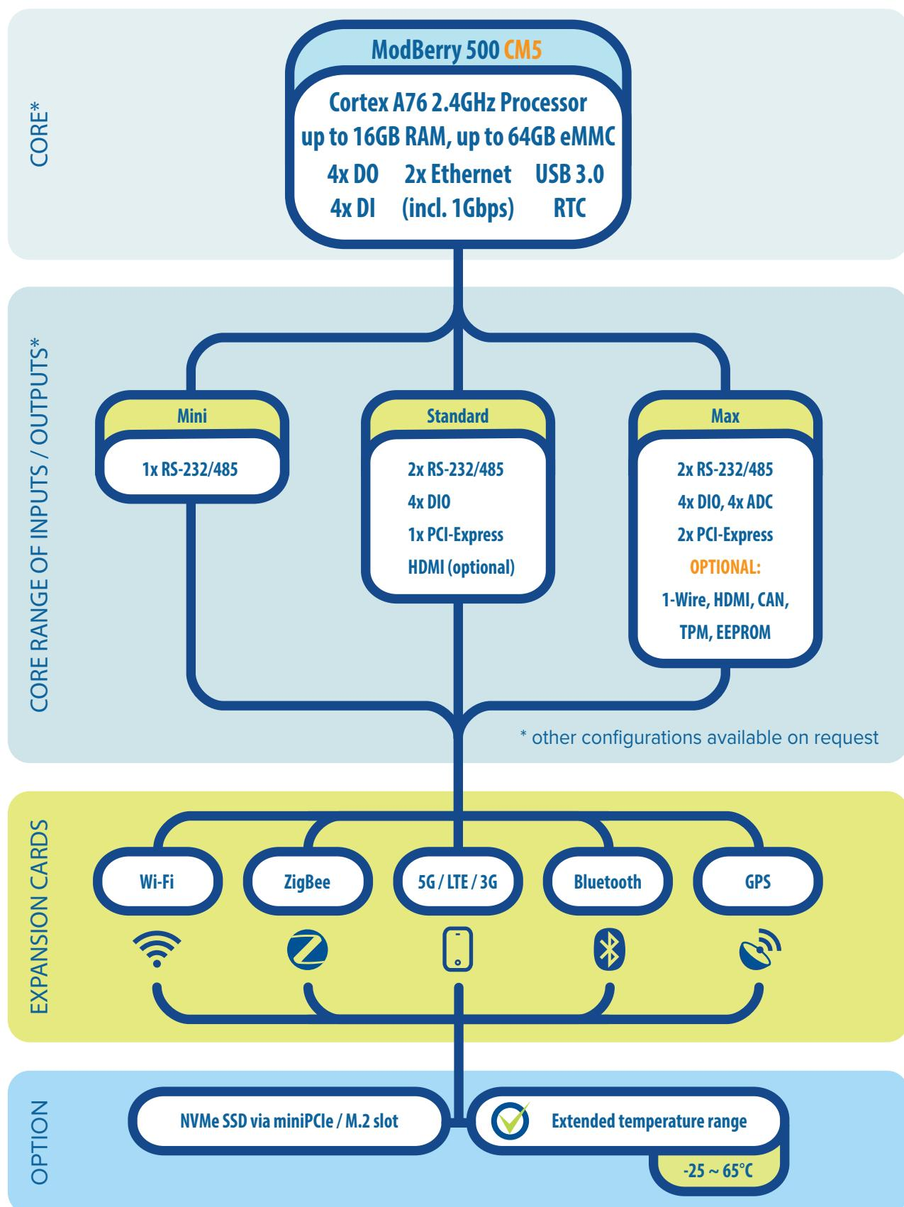
The **ModBerry 500 CM5** device allows use of up to 3 expansion modules, increasing its capabilities with additional I/Os, providing support for additional modems and wireless communication modules, and adding new features such as accelerometer and opto-isolation.
