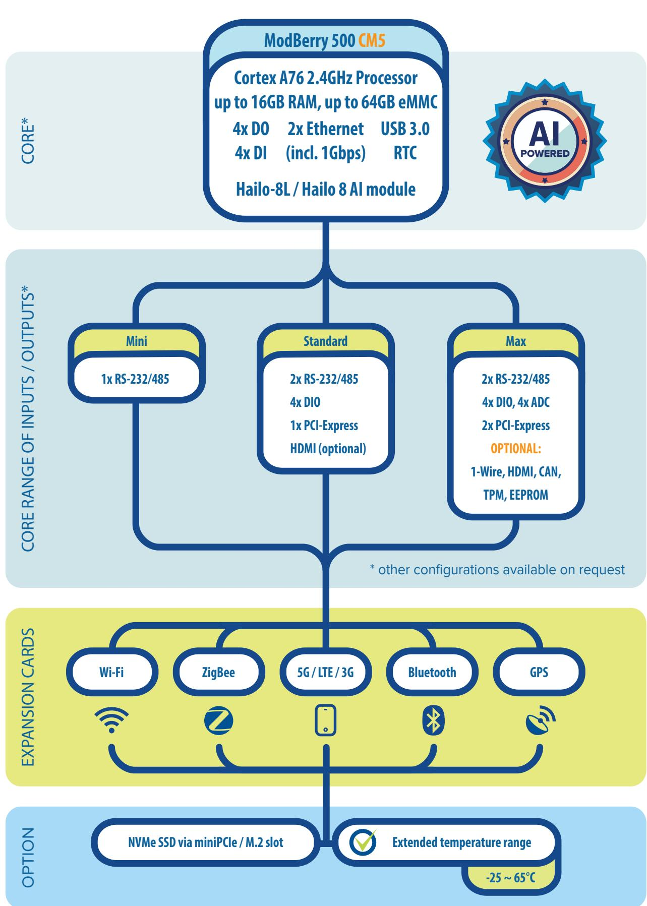
The **ModBerry 500 CM5** device allows use of up to 3 expansion modules, increasing its capabilities with additional I/Os, providing support for additional modems and wireless communication modules, and adding new features such as accelerometer and opto-isolation.
